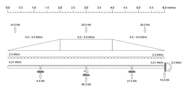
$Section: RMD \ Kwikform \ SuperSlim \ Soldier$   $Bending \ Stiffness, \ EI = 4020 \ kNm^2 \quad Shear \ Stiffness, \ GA = 17350 \ kN \quad Self-Weight, \ w = 0.210 \ kN/m$   $Self-Weight \ is \ included \ in \ the \ analysis \ with \ Partial \ Safety \ Factor \ 1.00$
